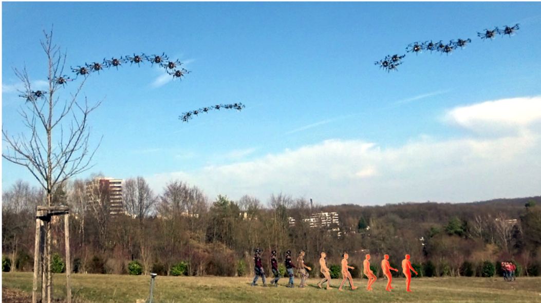
Figure 1: 3D markerless motion capture from fully autonomous micro aerial vehicles (MAVs) with on-board cameras. Multi-exposure image shows the trajectory of the MAVs and the 3D body pose and shape projected onto an image frame from an external camera. This camera was not part of the motion capture setup. Hence this camera, the MAV’s cameras, body pose projection and alignment were manually time synchronized.
